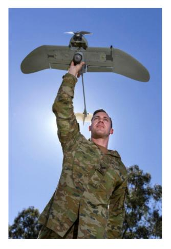
AeroVironment Wasp® AE Unmanned Aircraft System Selected by ADF (Image Courtesy of Australian Defence Force)
