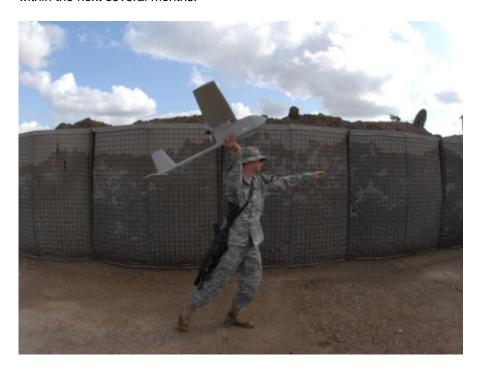
The Raven unmanned aircraft is a 4.2-pound, backpackable, hand-launched sensor platform that provides day and night, real-time video imagery for "over the hill" and "around the corner" reconnaissance, surveillance and target acquisition in support of tactical units. (Photo: Business Wire)
