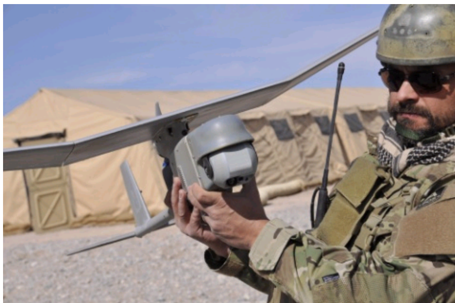
RQ-11B Raven with new miniature gimbaled sensor payload (Photo: Business Wire)
