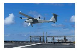
**THE JUMP** 20<sup>®</sup> is a vertical takeoff and landing (VTOL), fixed-wing unmanned aircraft used to provide advanced multi-sensor intelligence, surveillance, and reconnaissance (ISR) services. Delivering 13+ hours of endurance and an operational range of 185 km (115 mi), the JUMP 20 is ideal for multi-mission operations. Runway independent, the system can be set up and operational in less than 60 minutes without the need for launch or recovery equipment.
