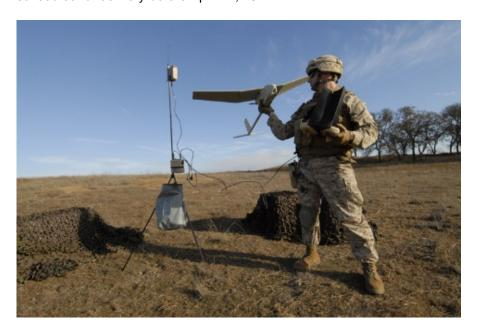
The RQ-11B Raven unmanned aircraft system is a 4.2-pound, backpackable, hand-launched sensor platform that provides "over the hill" and "around the corner" reconnaissance, surveillance and target acquisition in support of tactical units. (Photo: Business Wire)
