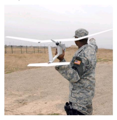
The Raven unmanned aircraft is a 4.2-pound, backpackable, hand-launched sensor platform that provides day and night, real-time video imagery for "over the hill" and "around the corner" reconnaissance, surveillance and target acquisition in support of tactical units. (Photo: Business Wire)
