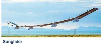
Ultra-long endurance solar-powered stratospheric unmanned aircraft - cruise altitude of 60,000 Feet
