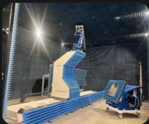
Automated RF Anechoic Chamber
