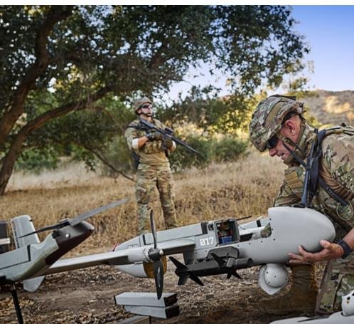
P550 autonomous eVTOL UAS transitions seamlessly from vertical launch to forward flight, carrying a multi-sensor payload. (Photo: AeroVironment)
