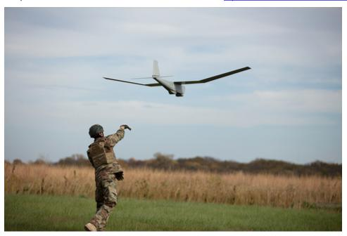
AeroVironment's PS2500 battery provides Puma 3 AE unmanned aerial systems users with up to three hours of continuous flight operations. (Photo: AeroVironment)
