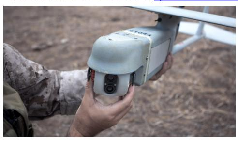
The Mantis i23 D daytime imaging payload system allows operators to capture ISR at a greater aircraft standoff distance without compromising image quality. (Photo: AeroVironment, Inc.)
