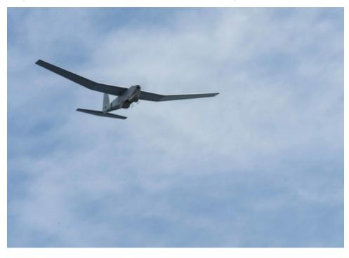
The Puma 3 All Environment (AE) unmanned aircraft system operates autonomously, providing persistent intelligence, surveillance, reconnaissance and targeting data (U.S. Navy photo by Mass Communication Specialist 3rd Class Bill Dodge/Released). Disclaimer: The appearance of U.S. Department of Defense (DoD) visual information does not imply or constitute DoD endorsement.
