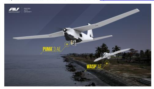
The Puma 3 AE and Wasp AE systems provide operators with reliable, on-demand tactical intelligence, surveillance, and reconnaissance and combine hand-launch capabilities with a deep-stall landing for operations in confined areas on land or water. (Image: AeroVironment, Inc.)
