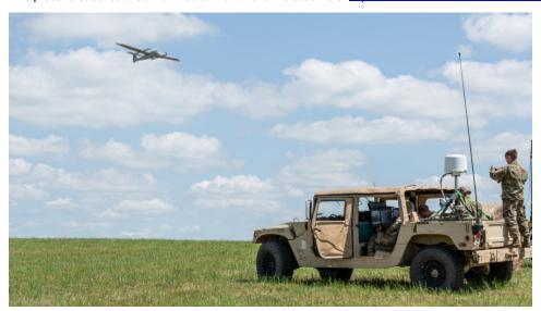
JUMP 20 is a VTOL, fixed-wing unmanned aircraft system that can be deployed quickly and requires no launch equipment or runway. (Photo: AeroVironment, Inc.)
