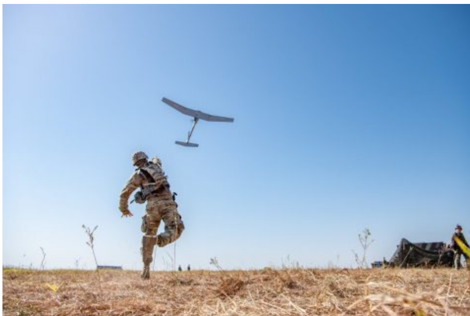
A U.S. Army Soldier hand launches a Raven B UAS in order to have a birds-eye view of the area during a field training exercise at Fort Sill, OK. (Photo: U.S. Army photo by Sgt. Dustin D. Biven)
