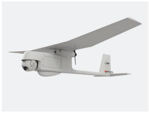
AeroVironment's Raven unmanned aircraft system is lightweight and rucksack portable, designed for rapid deployment to deliver real-time tactical situational awareness. (Photo: Business Wire)
