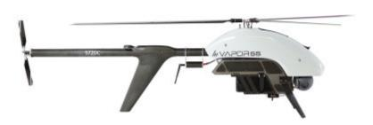
AeroVironment VAPOR 55 Helicopter UAS with Drop Mechanism and gimbaled EO/IR camera (Photo: AeroVironment)
