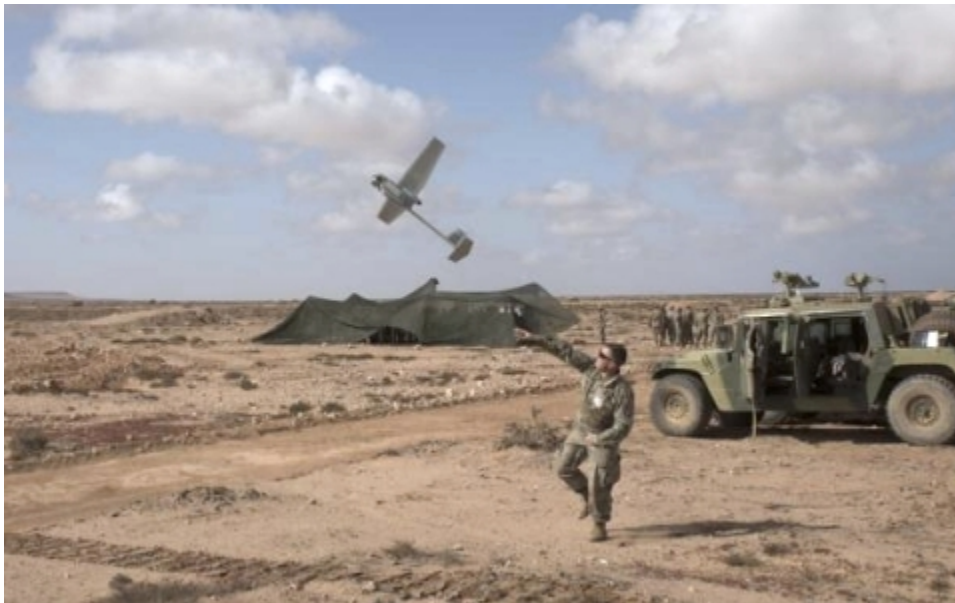
AeroVironment RQ-11B Raven Small Unmanned Aircraft System designed for land-based operations (Photo: Tech. Sgt. John Winn)
