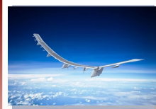
2019 HAWK30 Next generation solar HAPS for global connectivity and defense
