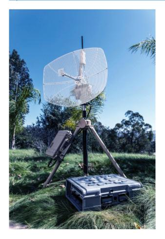
AeroVironment's new long-range tracking antenna for its Puma<sup>™</sup> AE small drone lets warfighters gather surveillance data farther from dangerous hostile fire. (Photo: Business Wire)
