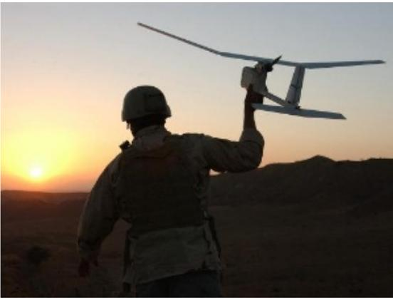
The Raven unmanned aircraft is a 4.2-pound, backpackable, hand-launched sensor platform that provides day and night, real-time video imagery for "over the hill" and "around the corner" reconnaissance, surveillance and target acquisition in support of tactical units. (Photo: Business Wire)
