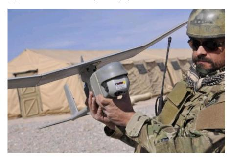
U.S. Army orders AeroVironment's RQ-11B Raven small unmanned aircraft system with its new multi-axis electro-optical and infrared video payload sensor (Photo: Business Wire)
