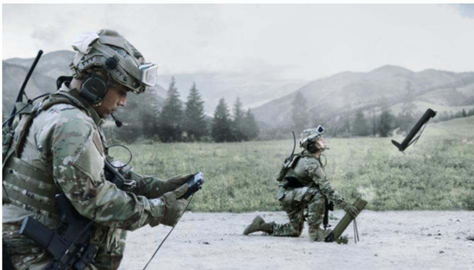
Switchblade 300 Block 20 is portable, lightweight, and easy to operate, requiring only a single operator. The new tablet-based Fire Control System allows operators to easily train, plan, and execute missions. Operation of the system is further simplified by offering an integrated control directly onto the launcher tube.
